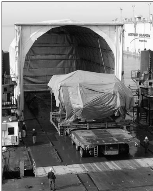
Above: A transporter loads the Auxiliary Machine Room (AMR) for North Carolina (SSN 777) on to a sea shuttle bound for General Dynamics Electric Boat in Groton, Conn., in February. Right: The 700-ton lower bow unit of George H.W. Bush is lowered into dry dock in March.
